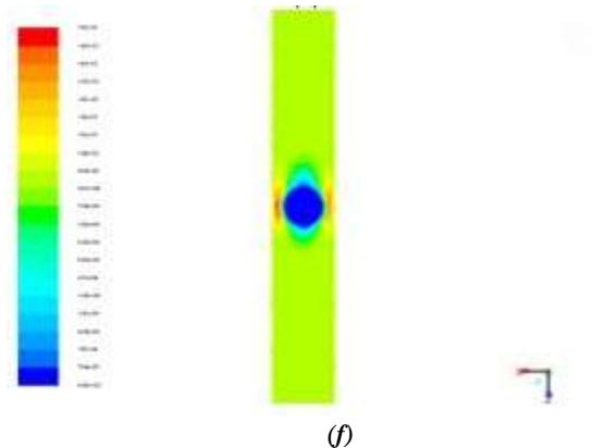
Figure (5): shown velocity profile contour for  $Re=10$  with different diameter ratio (a)  $B=0.1$  (b)  $B=0.2$  (c)  $B=0.3$  (d)  $B=0.4$  (e)  $B=0.5$  (f)  $B=0.6$
