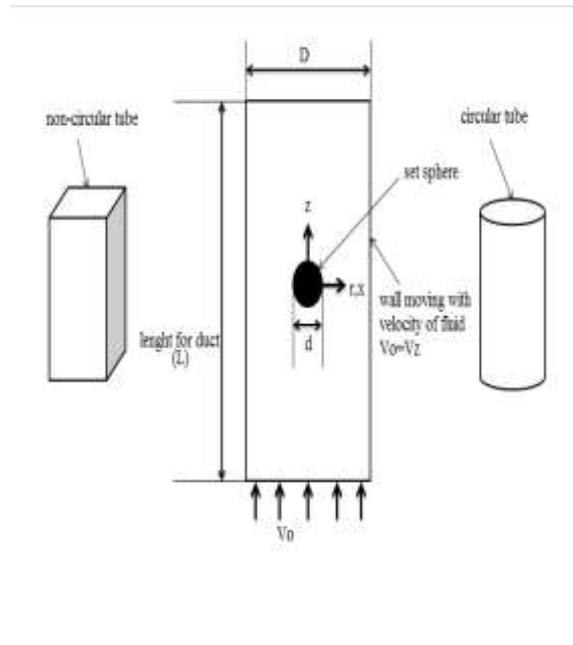
Figure (1): the flow around the sphere in circular and non –circular ducts.
