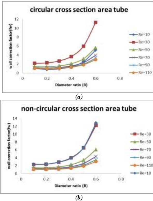
Figure (4): relationship between wall correction factor and diameter ratio in circular and non-circular tube (a) and (b).
